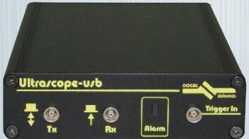
Ultrascope USB is the single-channel ultrasound system with highest performance in its market range. Its easy to use and intuitive software (ULTRAVIEW) includes all the functionality ( A-scan, B-scan ,C-scan, Peak detection,TGC,etc.) needed to take advantage of the equipment capabilities. The standard USB 2.0 connection along with its reduced
