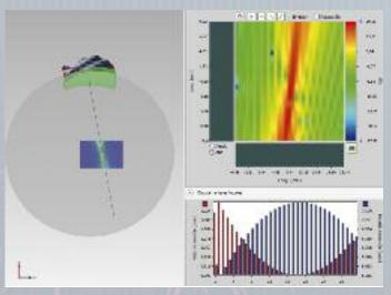
ultrasonic beam into the specimen. The obtained focal laws can be exported to SITAU systems or to other Phased-Array equipments that accept these input parameters.
