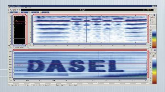
Its intuitive design reduces the learning curve, and so on, the time required to configure the equipment. Furthermore, it takes the maximum advantage of all functionality included in SITAU systems. For example: introducing wedge parameters, results presentation in all kind of views (A, B, C-scans) with measurement cursors of position, amplitude, attenuation and time-of-flight. Moreover, ScanVIEW includes a set of toolboxes for presenting, evaluat-
